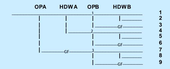
"GF" DENOTES SYSTEM FAILURE IF OPERATOR ACTION FAILS
